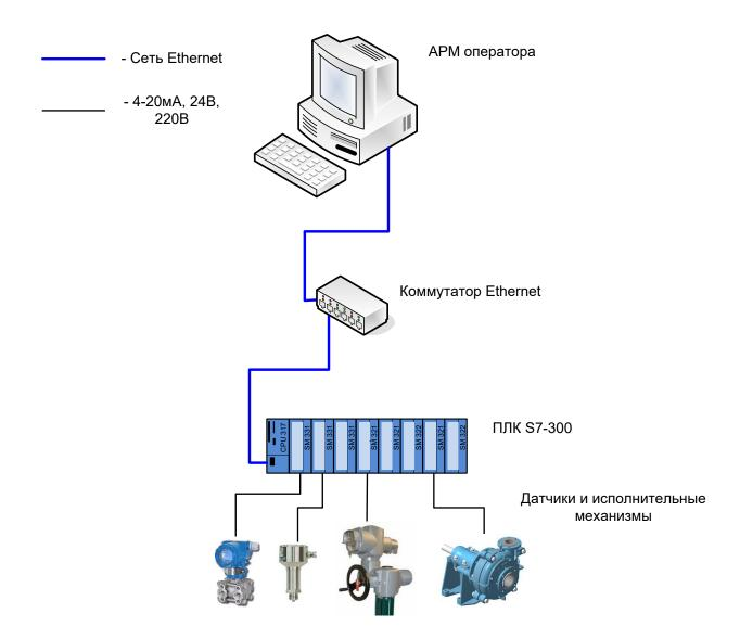
The automated process control system is divided into three levels. For a mini refinery, a block diagram of automation has been developed, see Fig. 3
