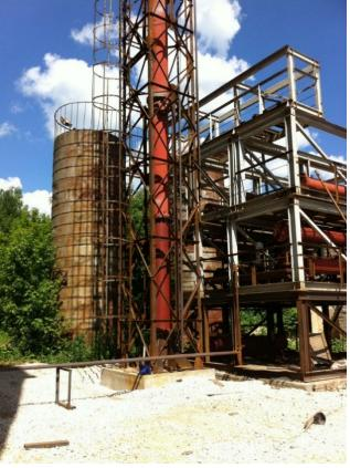
Technological facility -mini refinery has the following composition: -technological equipment (column, tanks, heat exchangers, pumps, valves, pipelines) which are interconnected with each other, in accordance with the technological scheme.
